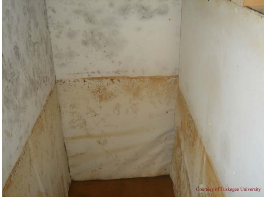
Figure 1.3 Flood Unit opened after three weeks showing mold development. Photograph Courtesy of Tuskegee University.
