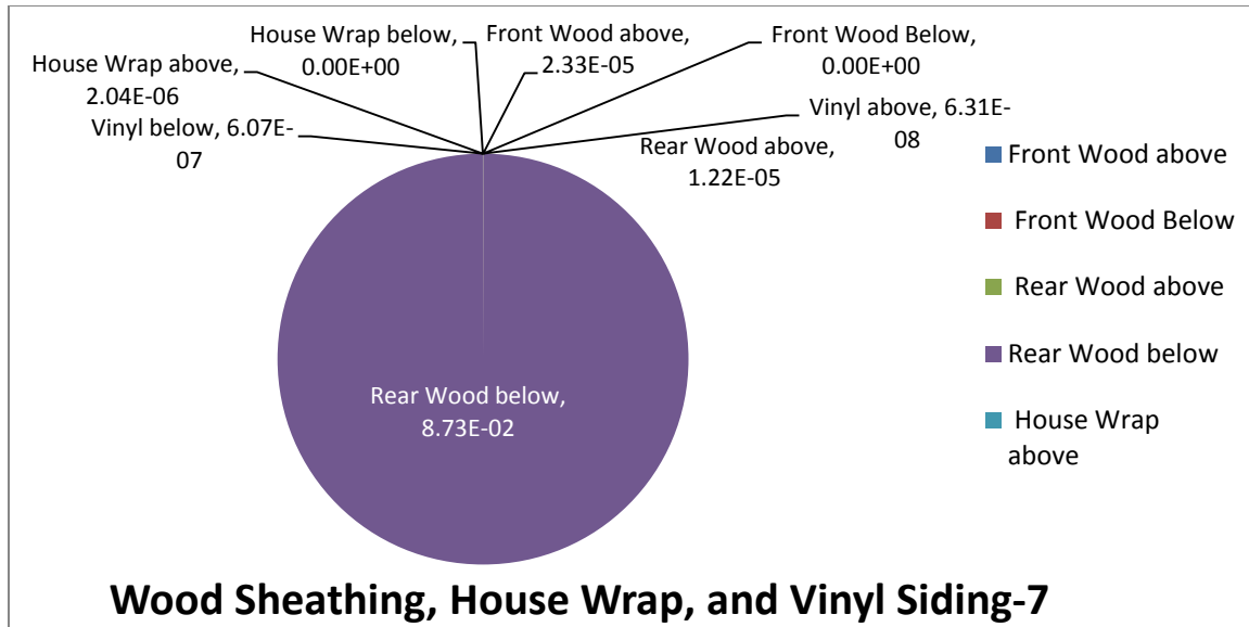
Figure 3.52 The distribution of Chaetomium globosum , based on DNA concentrations, on the wet wood sheathing, plus the house wrap, and vinyl siding-7 materials.
