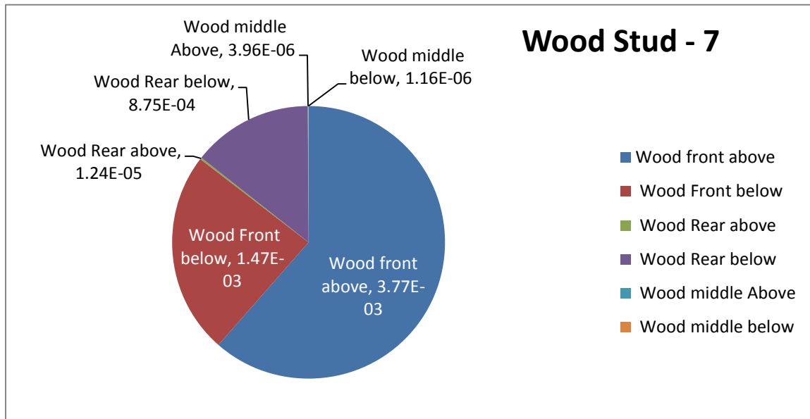
Figure 3.51 The distribution of Chaetomium globosum , based on DNA concentrations, on the different components of the wet wood stud-7.
